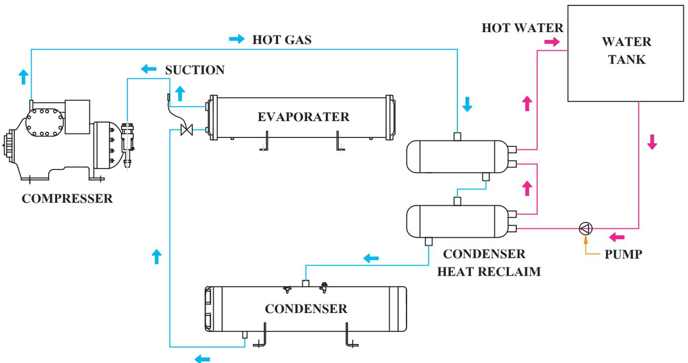
SELECTION SIZE OF CONDENSOR WHICH IS USED A HEAT RECLAIMER CALCULATED AT 30% - 50% OF CONDENSOR AND CHANGES SIZE OF INLET AND OUTLET REFRIGERANT PIPES INTO EQUAL TO HOT GAS PIPE.
